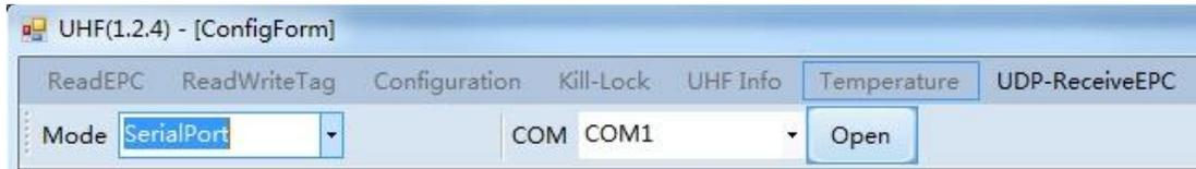
If RJ45 has been used as connection, communication **Mode** needs to be selected as “network” and input IP address and port number (default IP address is 192.168.99.202, Port is 8888.) Then click “Open” to connect PC and device. After PC and device have been connected, the status page is as follows:
